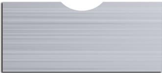
**Engraving:** The material is vaporized by the laser beam. The result is often a cone-shaped indentation due to the shape of the laser beam.
