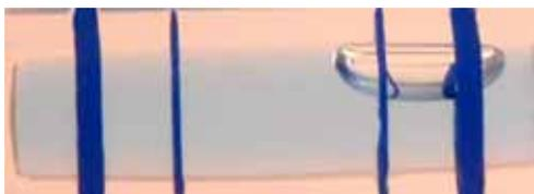
This photo shows an out of level condition. When the machine is level the bubble will be in the center of the two sets of lines.
