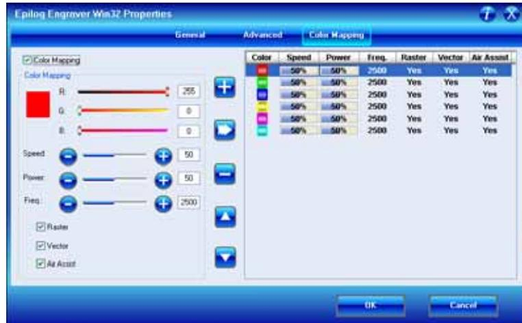
Make sure Color Mapping is checked so we can set up our color mapping scheme.
