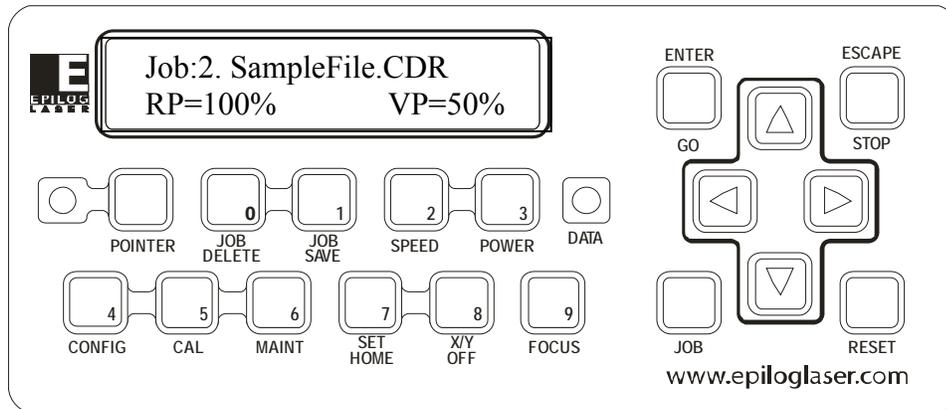
Pressing the **POWER** button while raster engraving will change the display to show the Power setting of the job while it is running (see diagram above). Pressing the **UP** or the **DOWN** cursor key will increase or decrease the power output of the laser in Raster Mode. Normally you will need to increase or decrease the Power by 10% or more before you start to notice a visible change. You cannot change Power on the fly in Vector mode.
