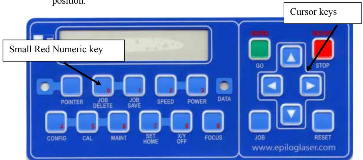
4. Press the **Right** cursor key on the keypad to advance the flashing cursor to the next set of three numbers (168 in our example).
