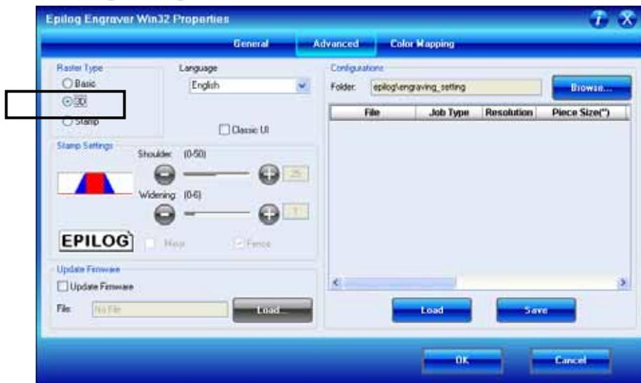
Earlier in the manual we discussed dot patterns and how those patterns are used to create raster images. 3D mode looks at the dots and the dot patterns in a very different way than Basic raster engraving mode, especially where it concerns either color, or grayscale images.
