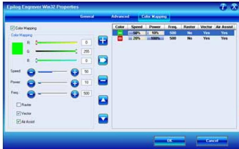
**Color Mapping Sequence** - When color mapping is used, it *always* cuts in sequence starting from the top color in the Map List and working down. In our example red will cut first and green second.
