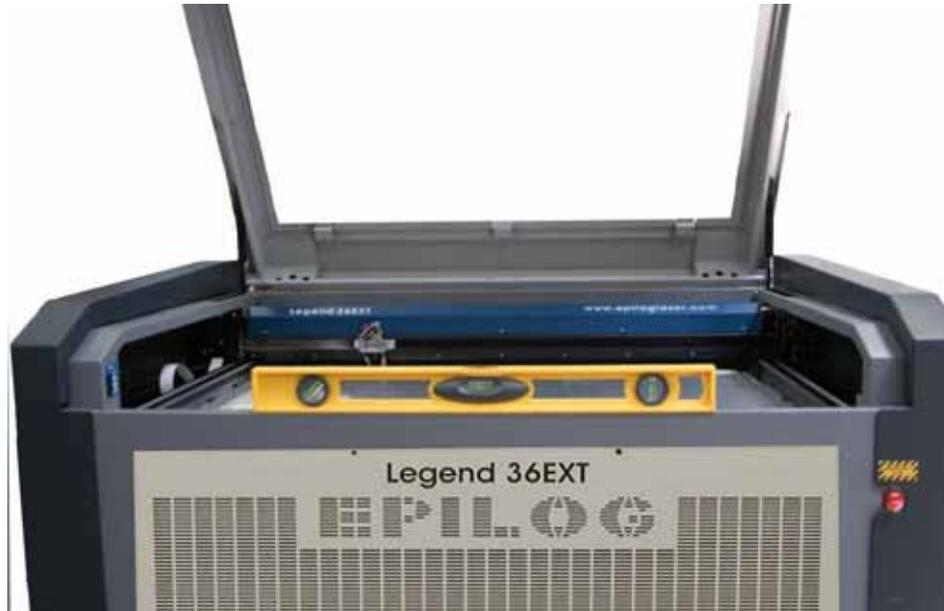
6. Locate the level's center indicator. The center indicator bubble shows the level of the machine.
