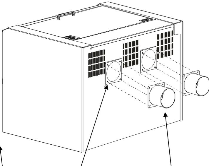
Mounting Screws (4 per port) - remove screws from chassis before installing exhaust ports.
