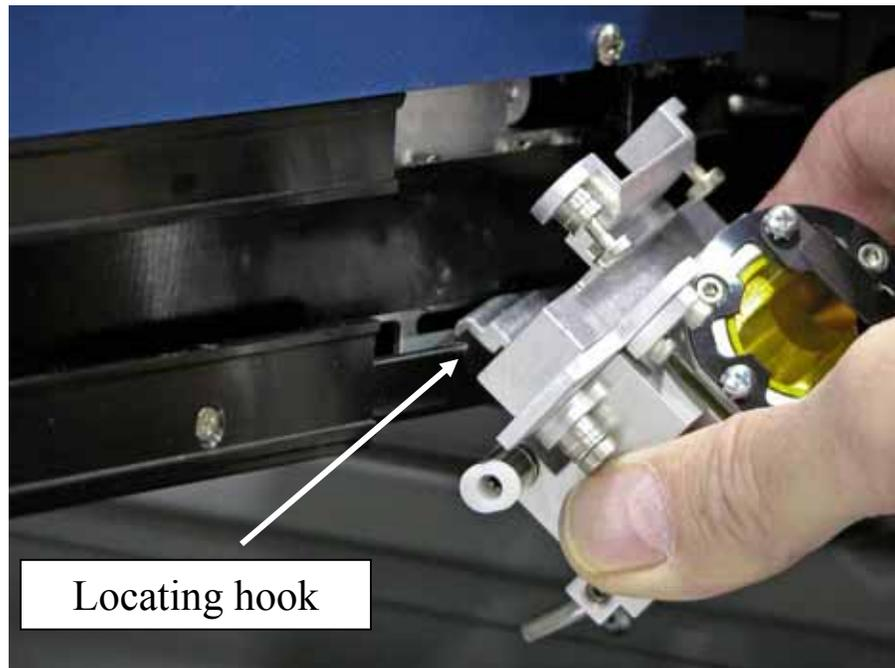
Insert the locating hook into the oblong slot in the secondary bearing block, and then rotate the top of the beam splitter/lens assembly up against the second bearing block. Secure the two Phillips head screws. If you feel resistance when attempting to tighten the two screws, unscrew them and make sure that the assembly is properly in place before trying to tighten the screws again.
