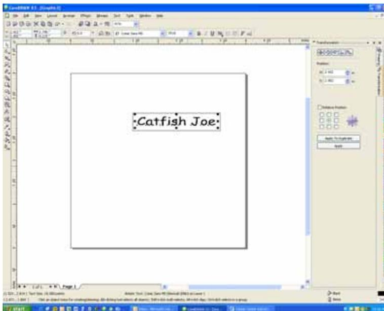
In this example we're going to use a small page that is 4" x 4" (102 x 102 mm). Create your artwork so that it is sized to fit into the available engraving area. In this example, we sized the text to fit within the available engraving area. 18 point text fits nicely into our box. Notice that the exact location of where you place the artwork is not important.
