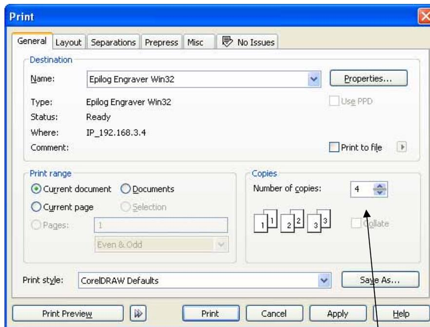
You can automatically engrave or cut a job multiple times by setting the Number of Copies to the number of passes that you want to make. When each pass is finished the laser will automatically start another pass until all passes are complete.
