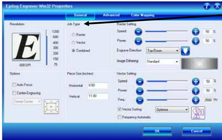
The Job Type: menu allows you to specify Raster, Vector, or Combined. This setting works in conjunction with the way your artwork is setup to produce a raster engraving, a vector profile, or a combination of the two modes in a single job.
