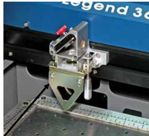
Place the manual focus gauge on the carriage. Use the **Focus** button and the **Arrow Keys** on the front control panel or the **Focus Key** inside of the laser cabinet to move the table up until your material just touches the bottom of the gauge. Once the focus position has been established, remove the gauge. Press the **Reset** button to return the carriage to its “Park” position before starting your job.
