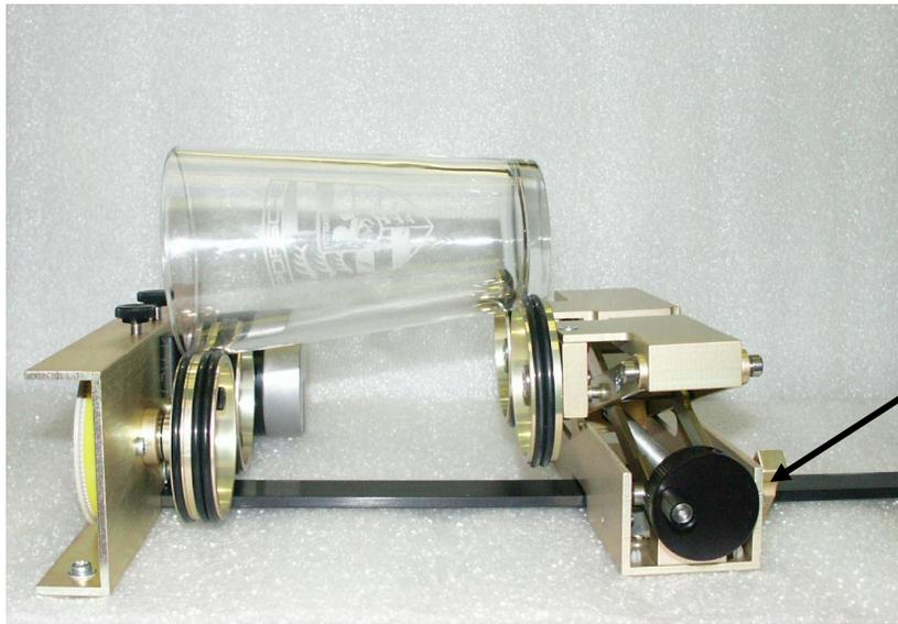
Use the elevator on the rotary attachment to raise the right side of the object being engraved so that its engraving surface is horizontal.
