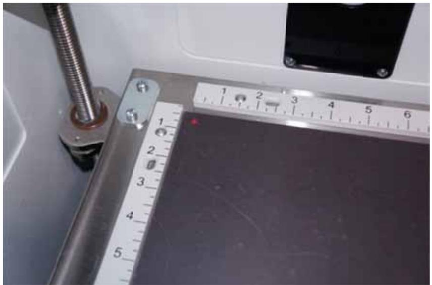
the bottom of the vector grid to these slots and press the vector grid firmly into the slots. You should feel a tactile “click” when the vector grid is properly seated.
