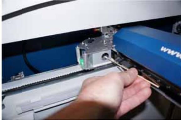
The photos below shows how to clean the focus lens. Remove the lens carriage from the machine to clean both the top and bottom of this lens.
