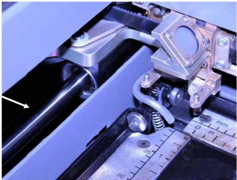
After cleaning the rails and bearings, clean off the table and the rest of the inside of the machine. Spending just a few minutes a week will pay off in the long run with better quality and performance.
