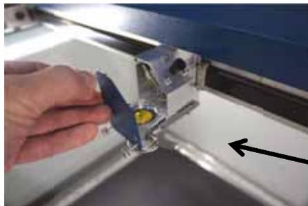
The crash bar is removed as part of the lens assembly. When reinstalling the lens assembly, please make sure that the Crash Bar is sitting on top of the locating pins on the side of the carriage. Crash Bar and locating pins.
