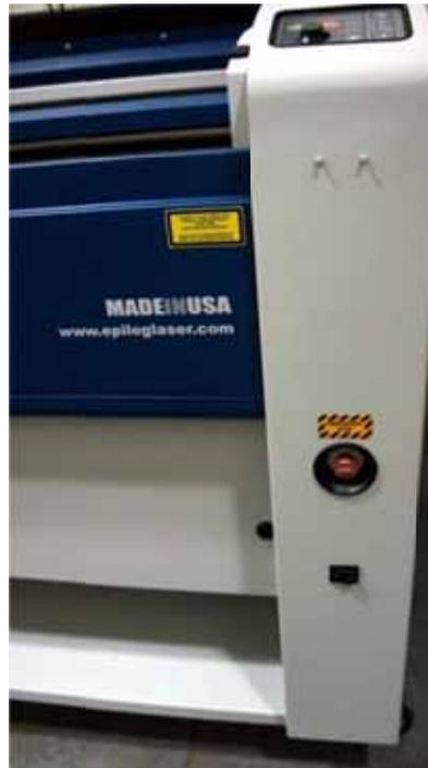
The emergency stop can be used to completely shut down the Fusion system in case of an emergency. If the emergency stop is used you will need to turn off the machine using the regular power switch, and then pop the E-Stop back out and then restart the Fusion as normal.
