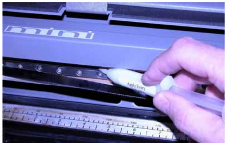
After applying the grease to both grooves, run the X-carriage over the grease to work it into the bearing block and rail.
