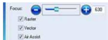
Change the slider in increments of Ten by clicking directly on the Plus or Minus icons. Each unit of 10 is equal to 0.010 inch (.254 mm). The screen below shows a focus setting of -500. This setting will move the table .500 inches (12.7 mm) closer to the focus lens.
