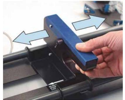
4. **Clamp your Cylinder:** insert your cylinder into the 3-Jaw Chuck and tighten the chuck so the cylinder is held firmly in place.
