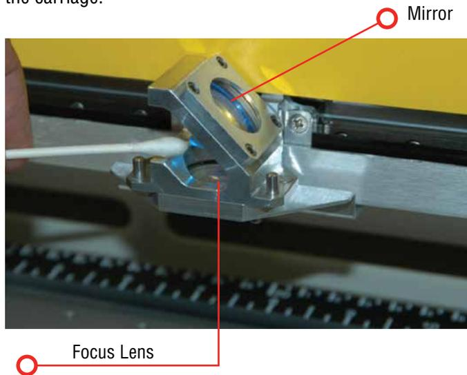
To clean the optics, use a high-quality cotton swab moistened with the optics cleaner supplied in the accessory kit. Please read the label on the bottle carefully.
