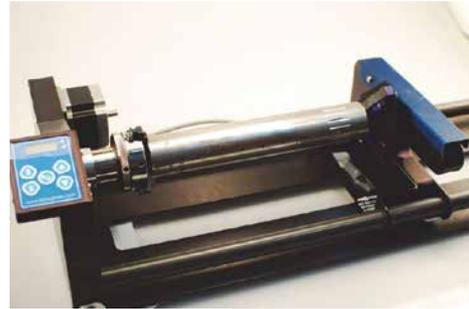
This photo shows a typical example of a larger part that requires a fixture plate on both the left and the right sides. Notice that the left side fixture plate is held in place with the 3-Jaw Chuck.
