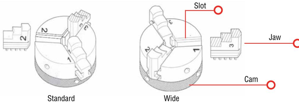
Pay particular attention to aligning the numbers as shown on the diagram when flipping the jaws! Failure to align the correct jaw in the correct slot will result in uneven spacing of the jaws when they are tightened.
