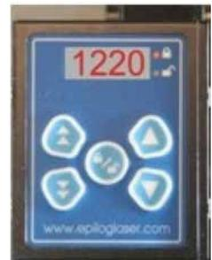
The display can show number in either inches or mm. The only indicator is if there is a decimal point showing on the display. A decimal indicates that the display is showing millimeters. To toggle between inches and millimeters, **press and hold the Lock/Unlock key** for several seconds until you see the display change. Once the display is set to the units you want, the Rotary Attachment will default to those units every time it is powered on.
