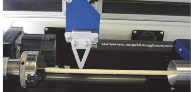
The 3-Jaw Chuck can be used with the standard 3" lens, or the optional 1.5" lens can be used to accommodate larger diameter pieces.
