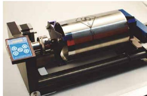
This photo shows the standard 3-Jaw Chuck on the left side and the idle-side centering fixture on the right. The idle-side centering fixture can accommodate sizes up to 1" in diameter.
