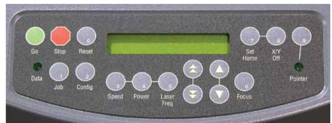
1. To set the IP Address, press the **Go and Pointer keys on the control panel at the same time**. You will see **FUNCTIONS MENU** displayed on the control panel LCD screen.
