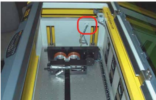
5. Once the Rotary Attachment is plugged in you can power on the system.
