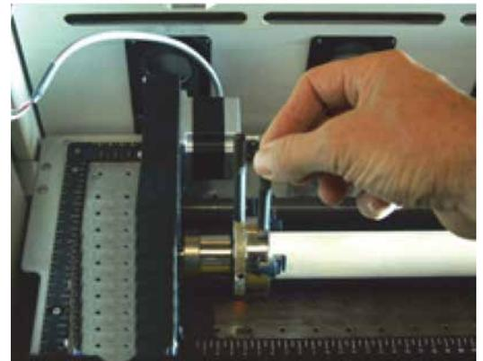
Cylinders can be held from the outside diameter or the inside diameter.
