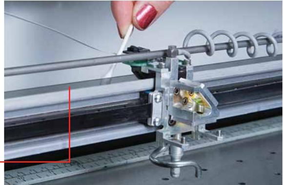
To remove the X-beam cover, turn off the laser and loosen the two screws in front of the cover and five in the rear of the cover. You do not need to remove the screws - they just need to be loosened to remove the cover. Lift the cover from the beam to expose the optical encoder and the optical strip.
