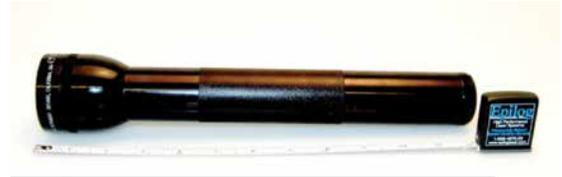
2. **Set the height of your page (in the Y direction) to the circumference of the cylinder you are engraving in the area where you will be etching.** Use a flexible tape measurer to find the circumference of the cylinder at its largest diameter. For this flashlight, the height of the page is 6" (152 mm).
