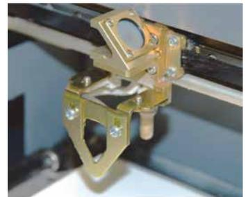
in the upper left corner of the machine. Press **Focus** on the keypad, then use the Up and Down Arrows to move the table to the correct height. Once the focus position has been established, remove the gauge. Press the **Reset** key.
