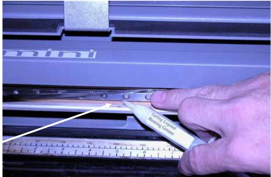
This photo shows the location of the X-axis carriage and the X-axis bearing (which is behind the X-axis belt).
