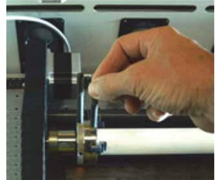
Cylinders can be held from the outside diameter or the inside diameter.
