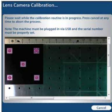
9. Once the Lens Camera Calibration routine has finished, the lens camera will be fully calibrated. Press the **OK** key and move on to the third step - calibrating the stitching offset.
