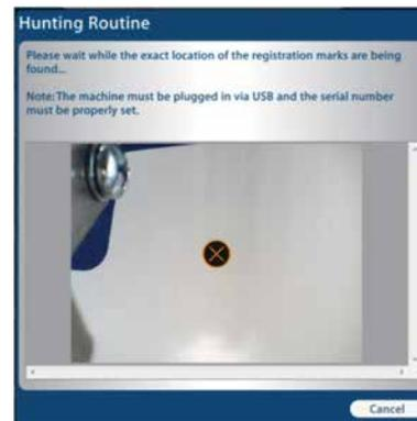
After locating the second mark, the carriage will stop moving while it is directly over the second mark. At this point, the vector files is transferred to the Fusion and the Fusion is ready to start cutting.
