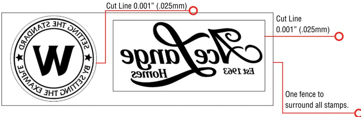
**Example 4: Incorrect!** The file contains multiple fence lines. If creating multiple stamps in one file, use one fence around the entire layout.
