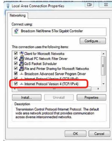
4. If you do not have an eView Camera Module installed, select **Use the following IP Address**. Type in the following IP Address: **192.168.3.3**.
