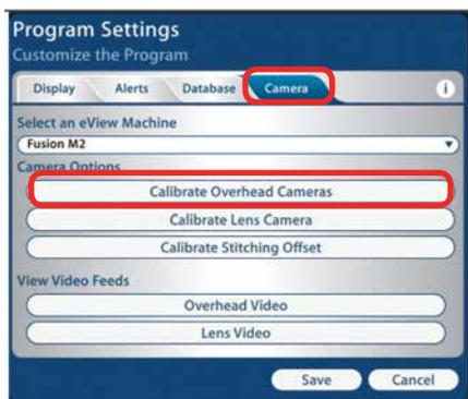
3. Select your laser from the drop-down menu, then click the **Proceed** key. The calibration routine will start immediately. The lens carriage will move across the bed left and right, from top to bottom, in order to map the entire Fusion table.
