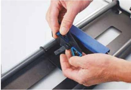
The splines on all the fixture plates can be reversed to accommodate parts using the inside diameter (ID) or outside diameter (OD). To reverse the spline orientation, pull the spring-loaded splines away from the plate and rotate them 180 degrees.
