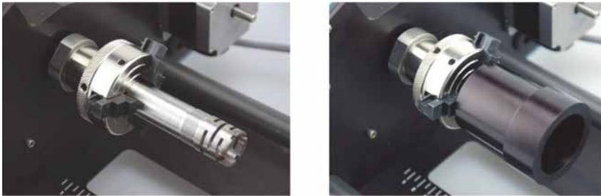
The chuck jaws can be flipped from Standard mode to Wide mode (180 degrees) to accommodate larger radius cylinders.
