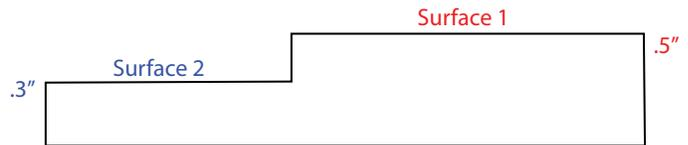
We will set up our artwork so that we engrave the Model Number on Surface 1 in red and the Serial Number on Surface 2 in blue. For this job, the only change we will make is to the Focus distance, everything else will be the same. In the Color Mapping tab you can see that we've set the red to a thickness of .5" (12.7 mm) and the blue color mapped layer to a thickness of .3" (7.62 mm).
