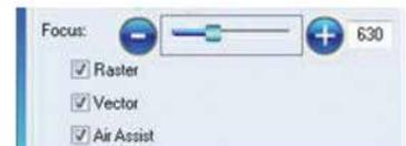
**Raster:** With this box checked, all raster objects set to that color will be processed at the color mapped settings; however, this function will still not allow a vector line set to a Vector stroke width to engrave.
