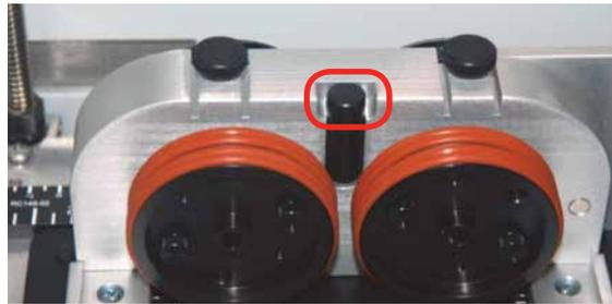
To establish the Rotary Home setting at the front of the black bumper we will use the Red Dot Pointer to show us where our Home Position is and then how far we need to adjust our settings. Once you have set and saved the X and Y Rotary Home Position you should not have to set it again.
