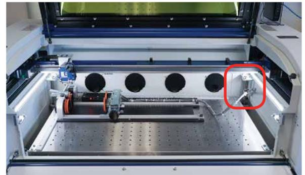
Once the Rotary Attachment cables are connected you can power on the laser system. The Fusion senses that the Rotary has been installed. During machine initialization the lens carriage will find its new Home Position over the center of the Rotary Attachment, as shown to the right.
