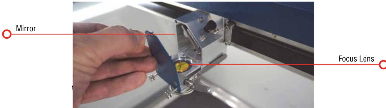
In addition to the focus lens and the mirror directly above it, there is a mirror located on the left side of the X-beam. This mirror is very well protected and should not need regular cleaning. It can be accessed with a cotton swab if it does need cleaning.
