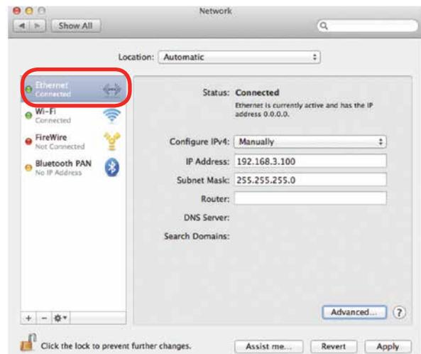
8. Select **Manually** for the Configure IPv4 setting, and then type in an IP Address that is different from the IP Address of your Fusion system.
