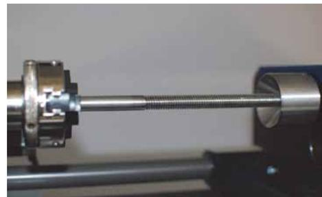
The centering fixture is used to support small diameter parts that sag when held in place using only the 3-Jaw Chuck.
