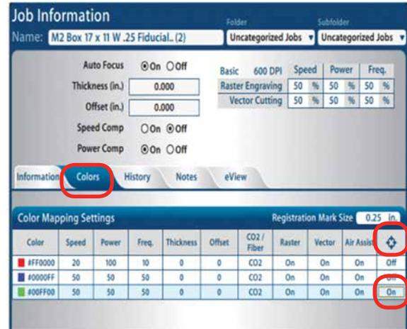
As soon as you click the Registration mark to ON the carriage will move as far back and to the left as it can go. This indicates that the Fusion is ready for the next step.
