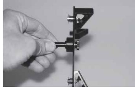
Slide the spindle into the chuck. Make sure the spindle is fully inserted into the chuck, then secure it using the chuck tightening pins.
