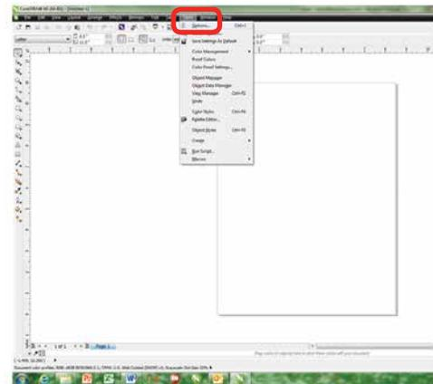
2. Under **Global > Printing**, choose **Driver Compatibilities**. Next to Printer choose the **Fusion Laser you just installed**. Check the box "**Send beziers and paths to driver**" and click **OK**.
