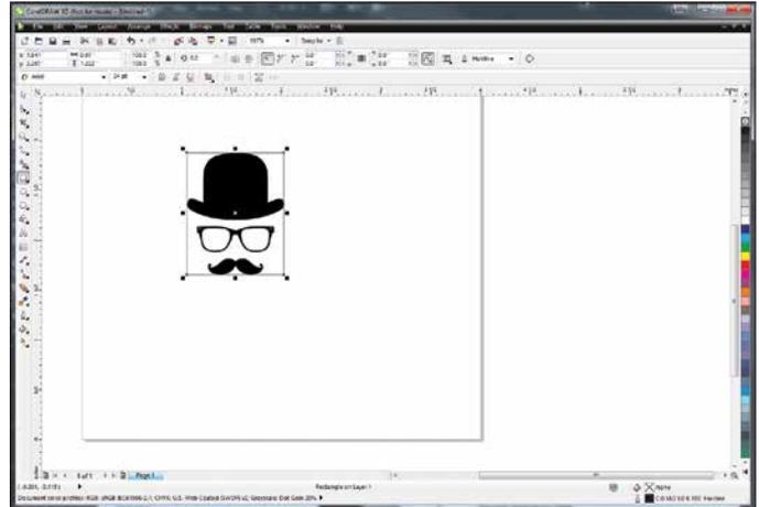
While Center-Center is the most common use for the Center Engraving features you can also use **Center-Left** and set a Home Position that is the left portion of your engraving area. **Center-Top** is at the middle, top area of the area you want to engrave. Depending on the object you are engraving, this may be easier to find than the center point of the engraving area.
