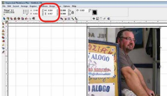
11. **Set the Resolution:** This number must match the resolution at which you will be engraving the photo. Select **Image** then **Image Size** from the menu. Type in the resolution and select **Apply**.
