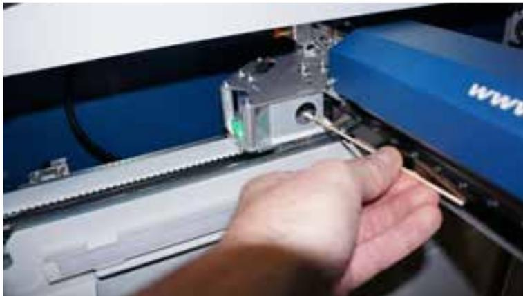
The photos below shows how to clean the focus lens. Remove the lens carriage from the machine to clean both the top and bottom of this lens.
