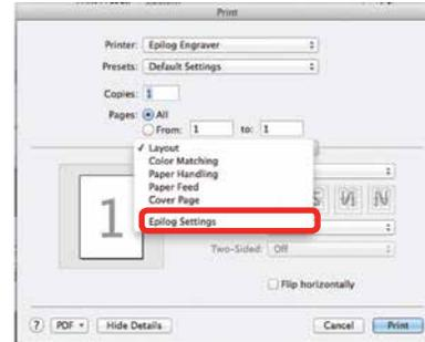
5. Set your laser **Settings**. We've set our Job Type to **Combined** because we'll be both engraving and cutting in this job. For Raster Settings, we've used **50% speed, 100% power**. For Vector Settings, we've used **30% speed, 70% power**. Finally, our resolution has been set to **600 DPI**.
