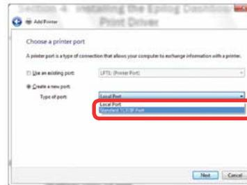
5. Enter the IP Address to match the IP Address you set at the Fusion laser in **“Setting the IP Address” on page 16**. Most Epilog users will use the IP Address of 192.168.3.4, which is what we use in this document. After typing in the IP Address, click **Next**. Wait while the computer identifies the port.
