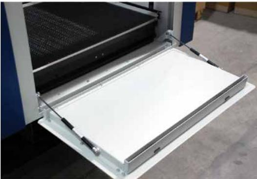
The front access door is usually used for easy loading and unloading of palletized materials. The door is interlocked and the laser will not fire if the door is open.
