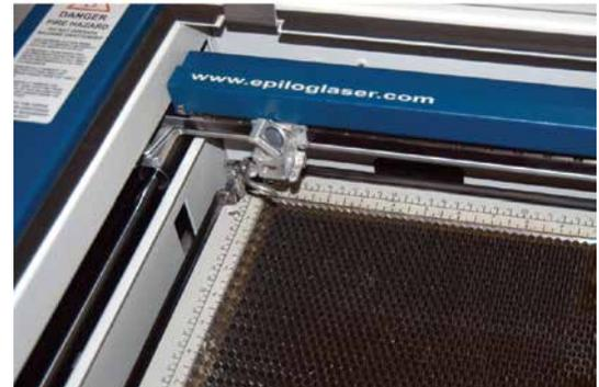
There is a leveling bar located below the vector cutting table that should always be in place to have the most level cutting table possible. To access the bar lift the rulers and remove the gridded table.
