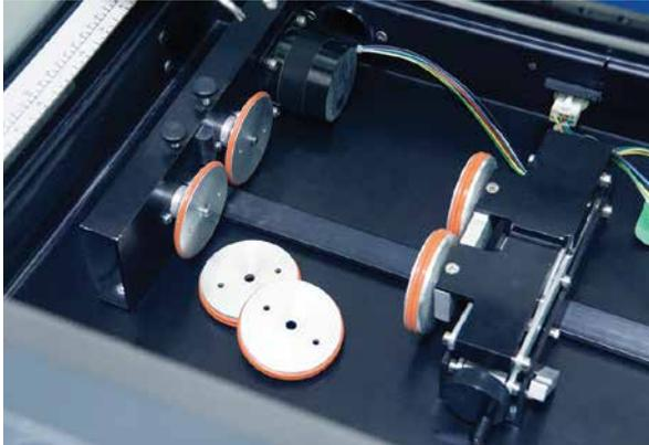
There are two small thumbscrews that attach each front drive wheel to the back drive wheel. Loosen the two small thumbscrews on each wheel to remove the front wheel.
