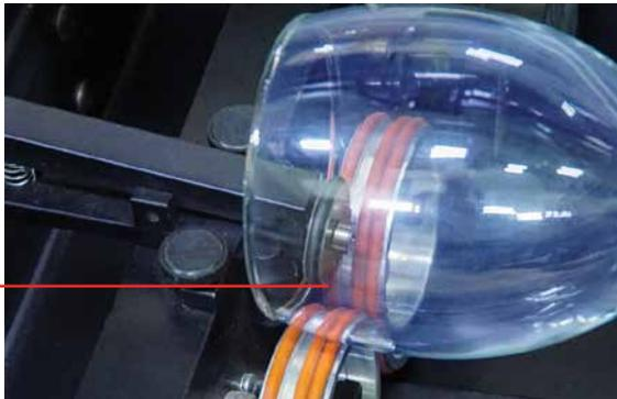
Many glasses, like this one, do not require the use of the clamp. The clamp is used mostly for hard to rotate cylinders or very lightweight objects that need more than just gravity to hold them in place.
