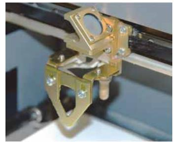
If your material has a taper or curve, pick an intermediate point between the highest and lowest points being engraved and focus on that point. In general, the area of the material being engraved needs to be relatively flat. If the area being engraved differs in height by more than about an .125" (3 mm), the image will begin to look "fuzzy" or out of focus.
