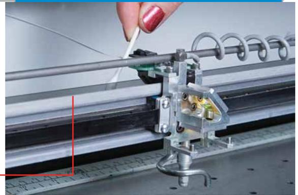
The encoder reader is a horseshoe shaped device that straddles the encoder strip. There is a possibility that dirt and debris can get inside the encoder. Blow some compressed air under the encoder to remove any dust and debris.
