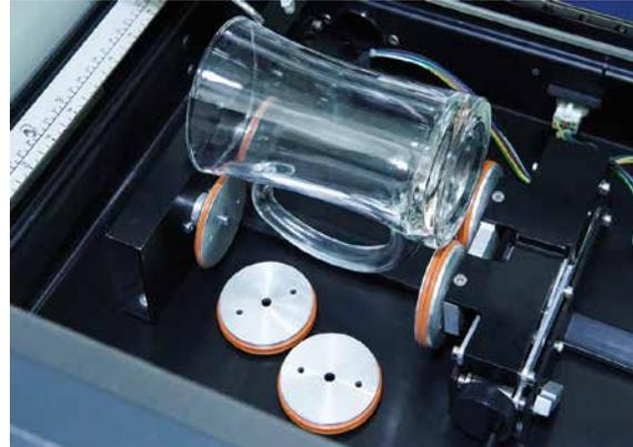
This photo shows a mug with a handle positioned on the Rotary Attachment with the removable portion of the drive wheel shown in the foreground.
