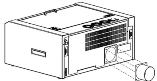
Once the exhaust ports are installed on the back of the laser system, use the flexible aluminum or galvanized sheet metal ducting to connect the laser system to the intake side of the exhaust fan. Then connect the exhaust side of the exhaust fan to the metal duct leading outside.
