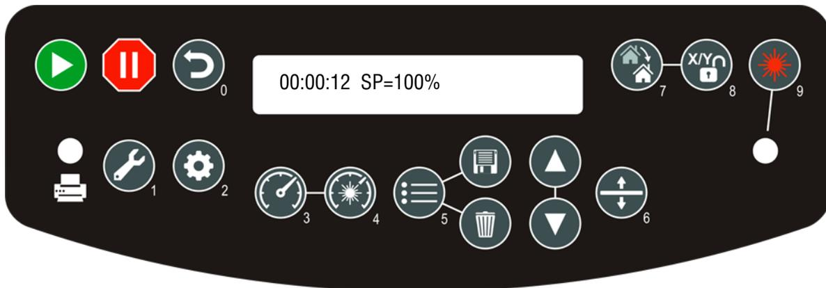
Pressing the Speed key while engraving will change the display to show the speed setting of the job while it is running (see image above). Pressing the Up or Down arrow key will increase or decrease the speed of the carriage. Normally you will need to increase or decrease the speed by 10% or more before you start to notice a visible change in the speed.
