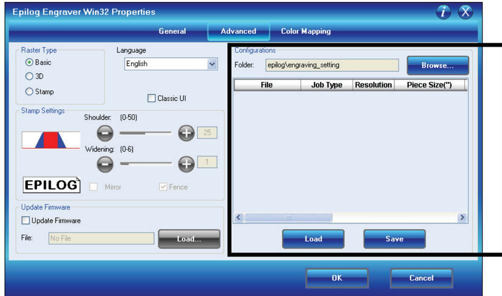
The “Configurations” feature is a comprehensive data management tool that is used to save all of your Dashboard settings for individual jobs. Saving the Dashboard settings as a database file allows you to retrieve the job parameters at a later time. This saves you the trouble of trying to remember what speed and power and other settings you used on a job you did three months ago. All of your settings can all be stored as a permanent record!
