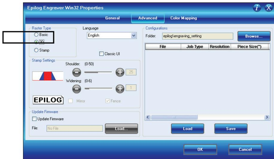
Earlier in the manual we discussed dot patterns and how those patterns are used to create raster images. 3D mode looks at the dots and the dot patterns in a very different way than Basic raster engraving mode, especially where it concerns either color, or grayscale images.
