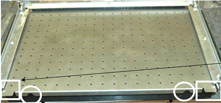
These tabs at the front of the task plate can be used to easily remove the task plate.
