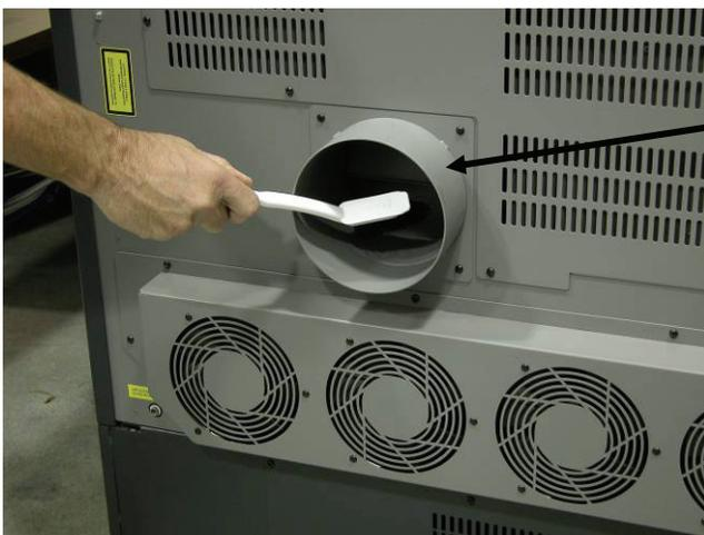
Periodically remove the duct from the back of the machine and clean both exhaust ports.
