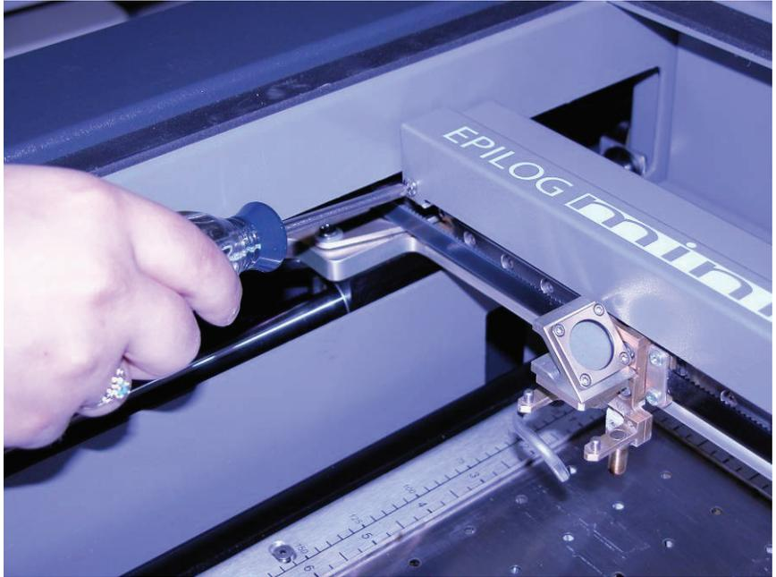
The X-beam with the cover removed. This photo shows the air assist tube and support.
