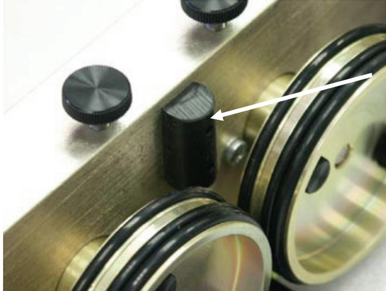
Set your glass on the rotary attachment so that it is close to this bumper, but not touching it. The glass may not be able to rotate freely if it is rubbing against the bumper
