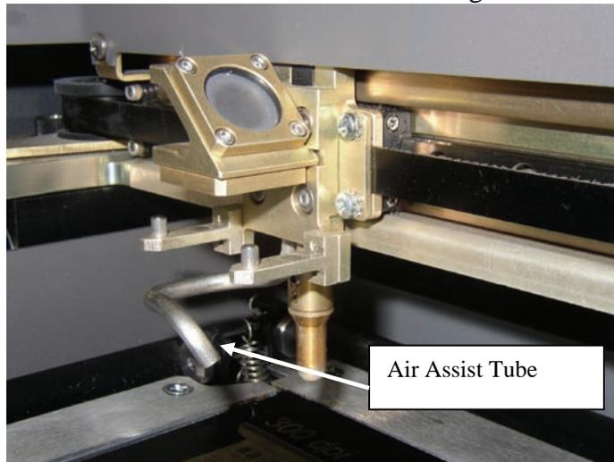
This photo at left shows the air assist tube. All Epilog systems have the plumbing for the air assist included (pump optional) as a standard part of the machine.
