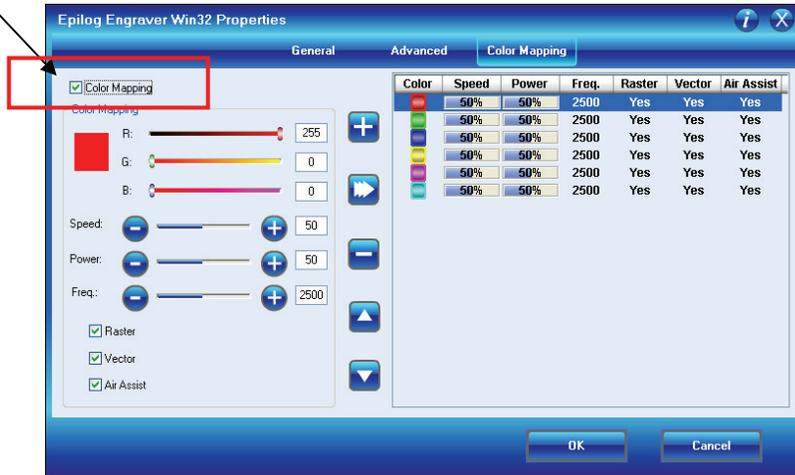
The Color Mapping feature is an advanced feature that must be checked to activate. While Color mapping is a very powerful tool, most users use it for two main reasons:
