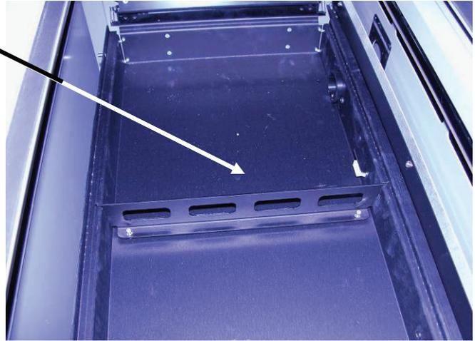
Once the task plate, vector grid, and insert are removed you will see three holes in the table tray that mate to the three pins in the bottom of the rotary attachment. Note that on the Mini 18 x 12 one hole is hidden in the cutout on the right side of the table.
