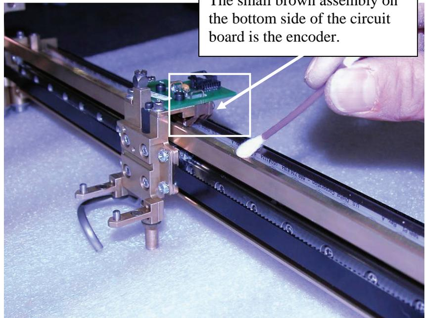
The small brown assembly on the bottom side of the circuit board is the encoder.
