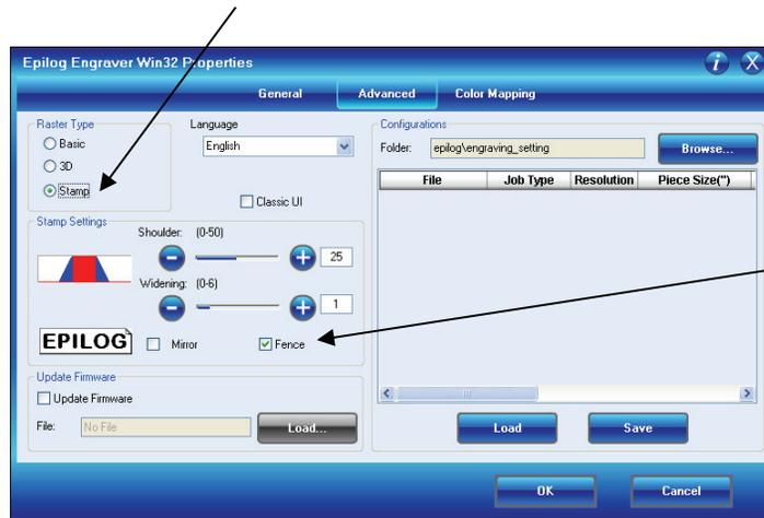
A check in the Fence box tells the engraver you are going to use a fence to define the area to be engraved away.
