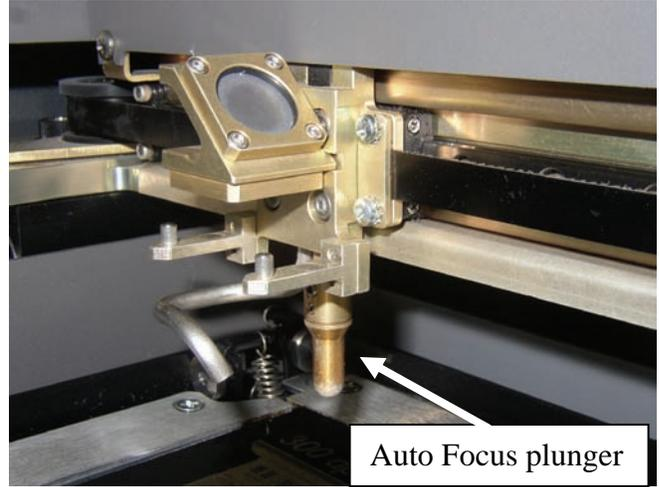
Checking the box will activate the Auto Focus process when the job starts to run.
