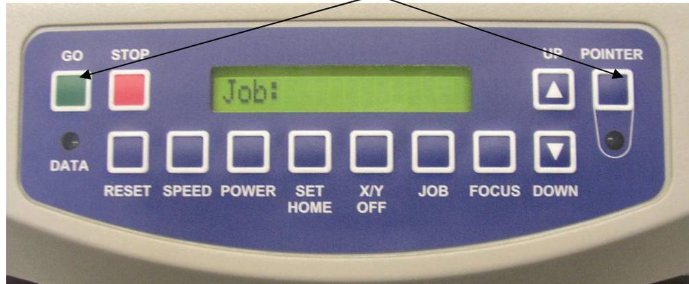
1. To set the IP Address press the **GO** and **POINTER** buttons simultaneously on the control panel. You will see “**FUNCTIONS MENU**” displayed on the control panel LCD screen.
