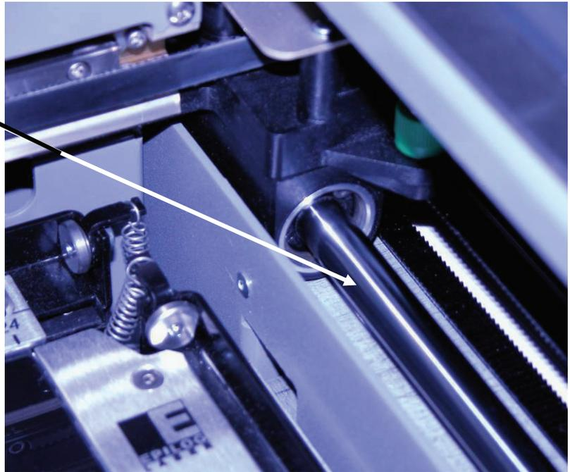
Clean the length of the left side Y-axis rail using a soft cotton cloth. Lubrication is not required.
