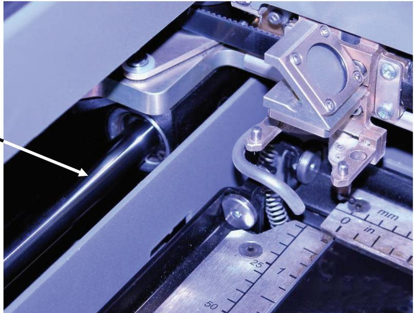
After cleaning the rails and bearings, clean off the table and the rest of the inside of the machine. Spending just a few minutes a week will pay off in the long run with better quality and performance.
