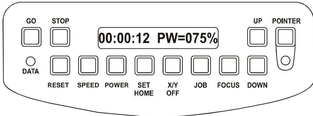
Pressing the **POWER** button while raster engraving will change the display to show the Power setting of the job while it is running (see diagram above). Pressing the **UP** or the **DOWN** key will increase or decrease the power output of the laser in Raster Mode. Normally you will need to increase or decrease the Power by 10% or more before you start to notice a visible change. You cannot change Power on the fly in Vector mode.
