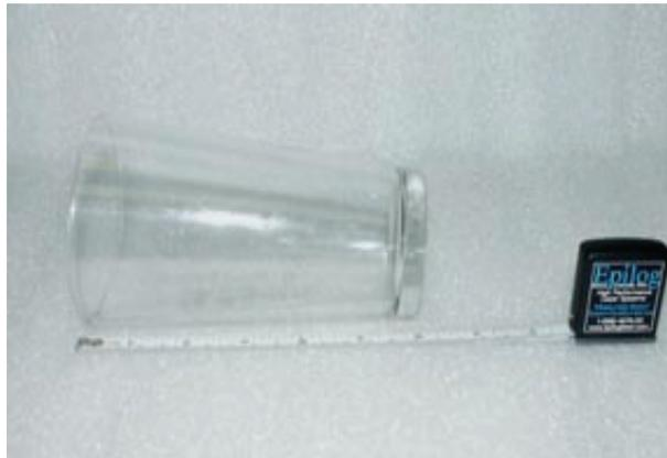
For the width (x-direction) of your page, lay the glass flat and orient it as it will rest on the rotary attachment. For this glass, the width of the page will be six inches (152 mm).
