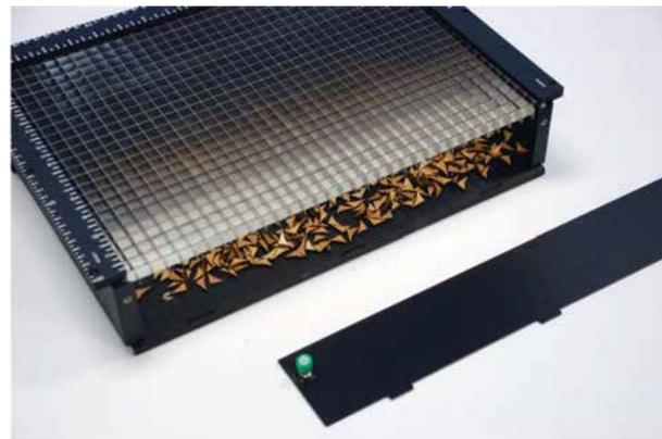
With the front plate removed, the Vector Grid can now be emptied of debris. Do not allow the debris to accumulate!
