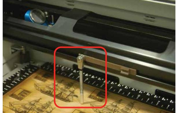
The photo below above the focus gauge that is built in to the X-beam of your laser system. You can move the focus gauge by hand from the far left to the far right side of the X-beam. This allows you to focus anywhere along the X-axis of the table. The focus spring will swing freely when released from its holder.
