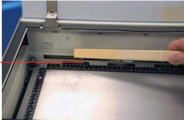
Periodically clean the exhaust plenum at the back of the laser. To access the plenum, remove the two small screws to the left and right of the exhaust port.
