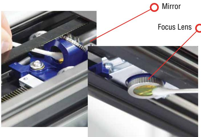
To clean the optics, use a high-quality cotton swab moistened with the optics cleaner supplied in the accessory kit. Please read the label on the bottle carefully.
