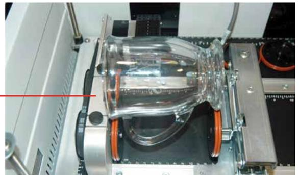
Use the scissor jack to raise the right side of the cylinder so that the engraving surface is horizontal. The photos below show the same flashlight at a severe angle to horizontal. If your cylinder is not horizontal to the X-beam, the laser will lose focus as the carriage head moves across the flashlight. This causes the engraving quality on the right hand side to suffer dramatically.
