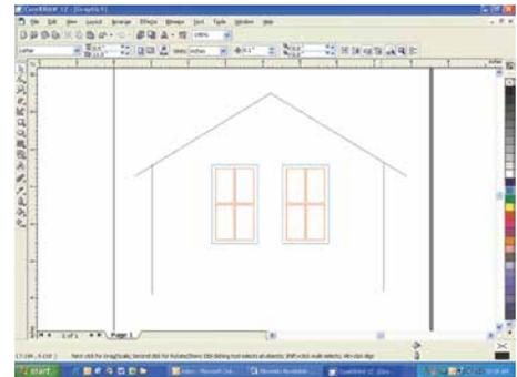
We have assigned the window frame vector line to the RGB green color, and the window panes to RGB red. You **MUST** use an RGB color scheme in your artwork with the Color Mapping feature. **CMYK values will not translate.**
