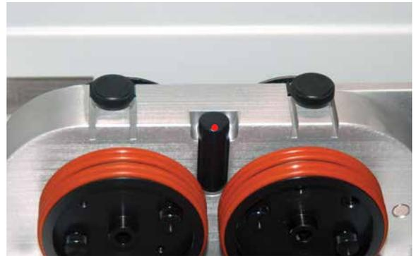
If your Red Dot Pointer is not at this location, you will need to adjust the X- and Y-axis settings to establish the correct Rotary Attachment Home Position. There is an adjustable numerical setting for both the X- and Y-axes that allow you to adjust your Red Dot Pointer so it is calibrated to the edge of the bumper. To change the rotary home settings, follow the instructions below:
