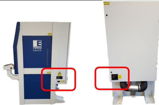
The primary On/Off switch is located on the side of the control panel. This switch is used on a daily basis for turning the G2 On/Off.
